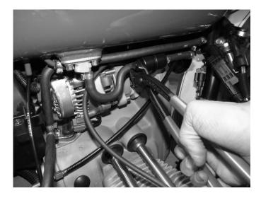
**Step 8**Install the new in-line fuel filter and replace all one-time use clamps.
