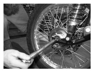
**Step 6**Position the wheel back on the bike and install the axle. DO NOT tighten fully at this point.
