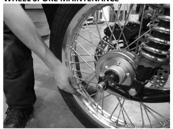
The wheel spokes should be checked on a regular basis as per the maintenance intervals.
