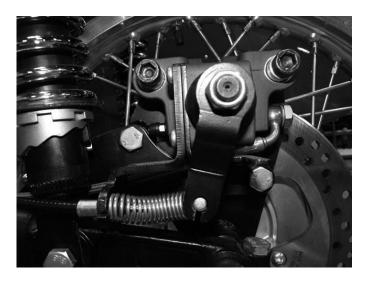
**Step 3**With the parking brake set you will have approximately 12mm between the caliper stop bracket and the brake are with spring.
