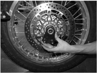
**Step 5**To re-install the wheel first place the caliper mount into the wheel.
