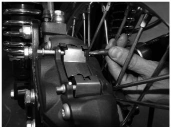
**Step 2**Carefully drive the retaining pins out of the caliper using a small punch or drift.
