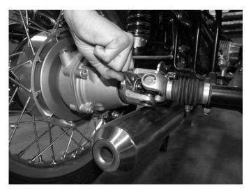
**Step 6** Remove the rear axle nut.
