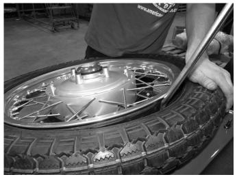
**Step 2**Using the provided tyre spoons in your tool kit carefully remove one side of the tyre from the rim.
