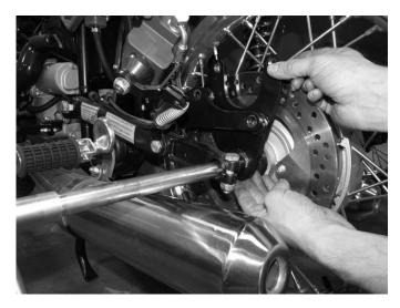
**Step 9**To re-install the rear wheel place the wheel back on the bike and push the axle through both the
