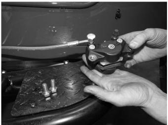
**Step 2** Remove the caliper from the sidecar swing arm.
