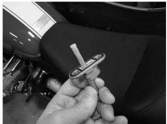
**Step 7**Clean all debris for the intake filter and re-install in the tank.
