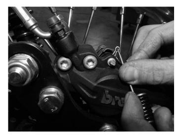
**Step 1** Remove the retaining pin safety clips.
