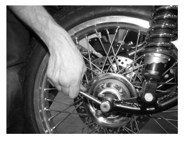
Loosen the axle by rotating clockwise and remove from the wheel.
