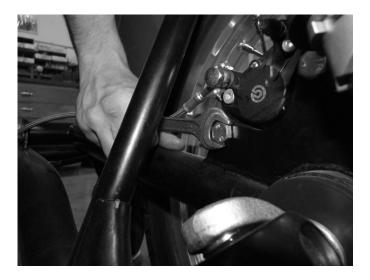
**Step 1** Remove the sidecar brake caliper.
