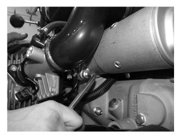
**Step 4**Loosen both the upper and lower starter bolts to allow clearance for battery removal.
