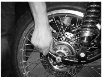
**Step 8**Tighten the axle by rotating counter-clockwise.
