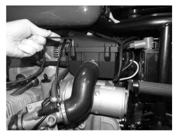
**Step 1**Remove the four retaining bolts form the air box lid using a 5mm hex wrench.
