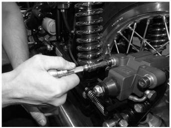
**Step 2**Remove the caliper retaining bolts.
