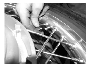
**Step 1**Remove the valve stem and deflate the tyre.
