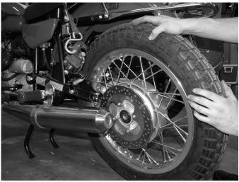
**Step 8**Remove the rear wheel by tilting the outwards towards you and rolling it back as shown.
