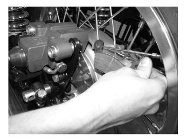
**Step 3**Remove the brake pads by pulling to the rear of the motorcycle.
