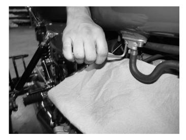
**Step 6**Remove the in-tank screen filter.
