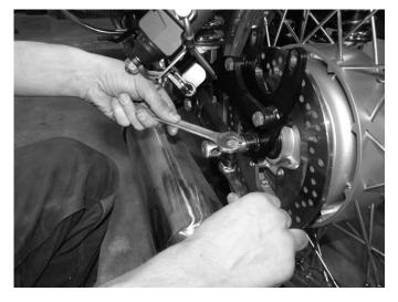
**Step 7**Loosen the axle pinch bolt and remove the axle.
