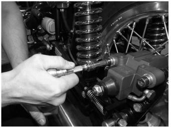
**Step 11**Re-install the brake caliper and brake pads.
