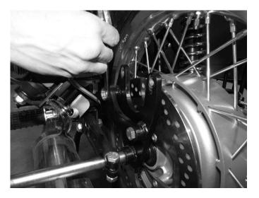
Torque the caliper mounting bracket bolts to specification.
