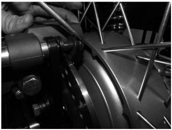
**Step 2**Carefully remove the caliper retaining bolt safety clips.
