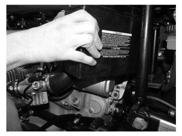
**Step 5**Carefully slide the battery out between the frame tube and air box.
