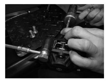
**Step 3**Remove the caliper safety clip and carefully drive the retaining pin out of the caliper with a punch or drift.
