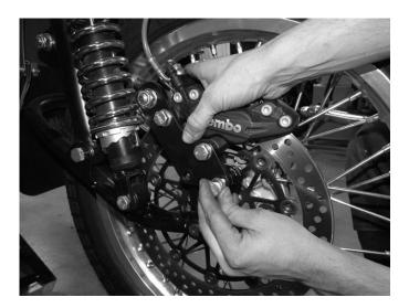
Re-attach the caliper with mounting brackets and tighten to specification.
