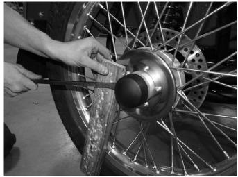
**Step 2** Carefully remove the sidecar hub cap.
