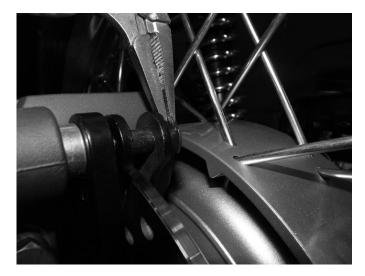
**Step 12**Re-install the caliper retaining bolt safety clips.
