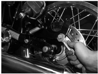
**Step 5**Remove the brake caliper mounting bracket bolts. Swing the support brace bracket up.
