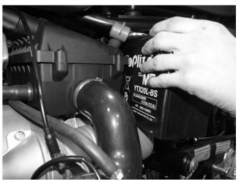
**Step 6**Re-install in reverse order by sliding the battery back into place and reconnecting all straps and cables.
