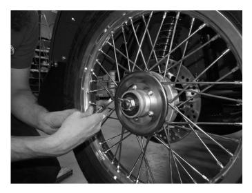
**Step 3**Remove the axle cotter pin and axle nut.
