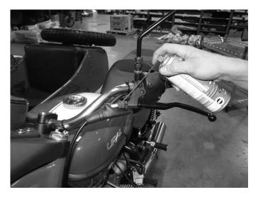
All cables including the clutch, speedometer, throttle, and parking brake cables should be lubricated with cable lube or WD-40 per the maintenance intervals. You should also lubricate all cables before and after extended periods of storage and/or after off road use.
