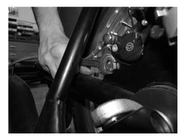
**Step 1** Remove the caliper mounting bolts.
