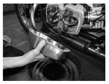
**Step 1**Starting with the left side cylinder, remove the valve cover and clean any contaminates found
