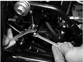
**Step 2** Adjust the cable to remove excess free play.
