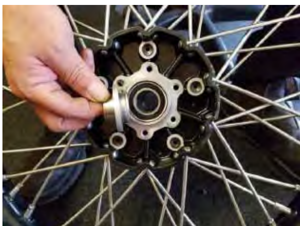
Remove the spacer and retaining ring
