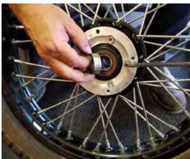
Remove spacer and disk holder from opposite side of spare wheel
